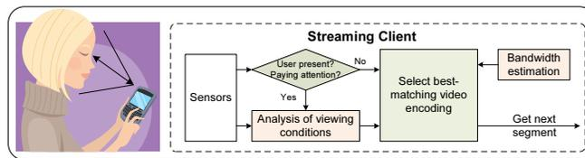
Figure 4. Illustration of functionality of DASH streaming client incorporating adaptation to user behavior and viewing conditions.
