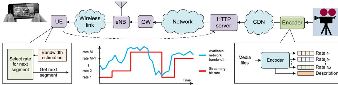
Figure 3. Illustration of functionality of mobile DASH-based streaming system. The multimedia content is encoded at multiple rates, and segmented in chunks allowing client to select portions that can be delivered in real-time, while also adapting to changing network bandwidth.
