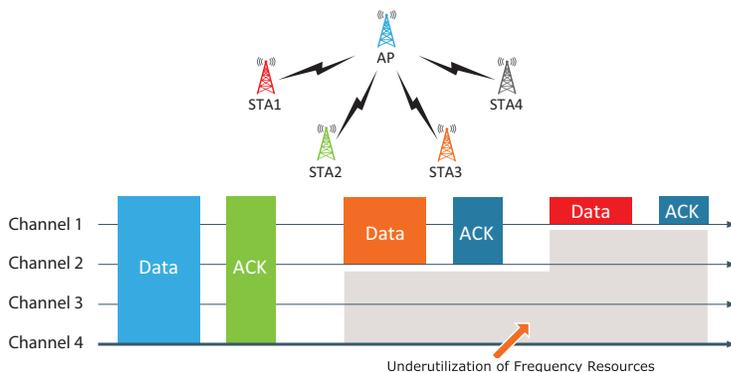
Figure 7: Inefficient Frequency Resource Utilization
