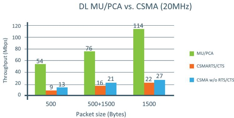
Figure 8: Efficient use of parallel frequency channels can provide 2x to 3x throughput improvement
