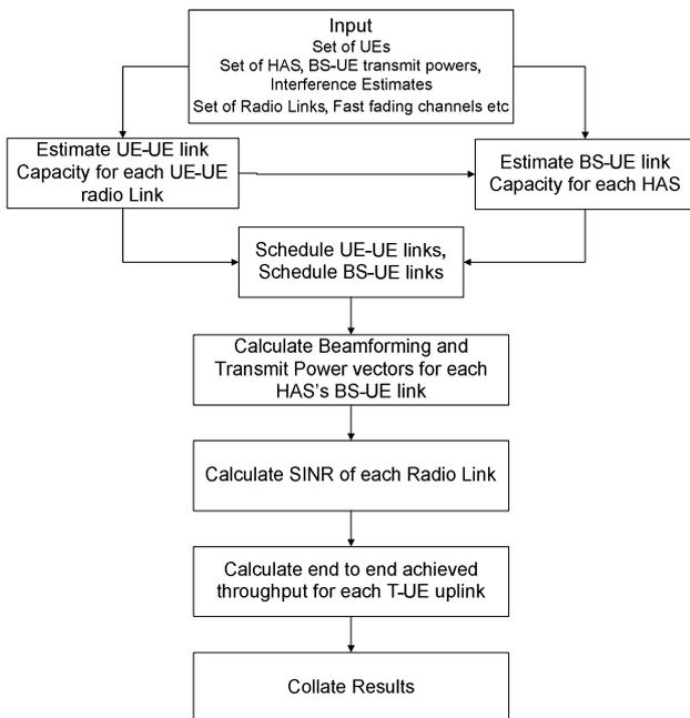
Fig. 4. System Simulation Flow Inner Loop
