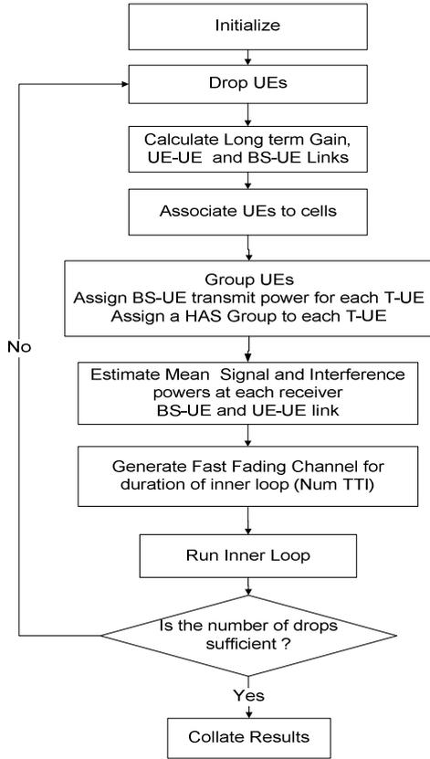
Fig. 3. System Simulation Flow Chart Overview
