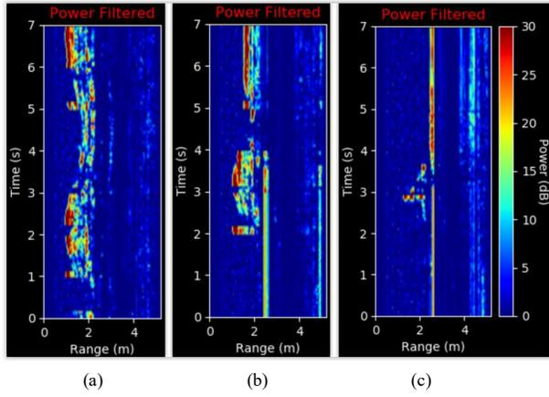
Fig. 4. Example of filtered range-time-power heatmaps of three indoor human activities for mmWave band after background subtraction. (a) Walking, (b) Sitting, and (c) Falling
