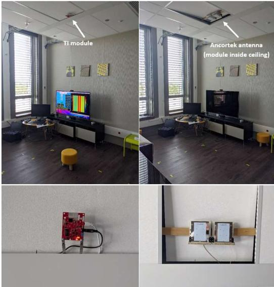
Fig. 1. Experimental setup with the two radar modules mounted on the room's ceiling
