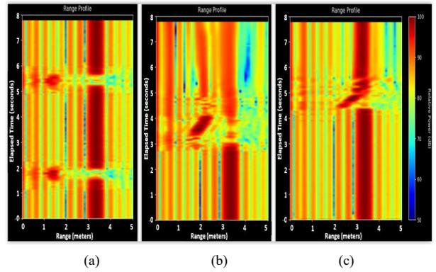
Fig. 3. Example of range-time-power heatmaps of three indoor human activities for sub-6GHz band. (a) Walking, (b) Sitting, and (c) Falling
