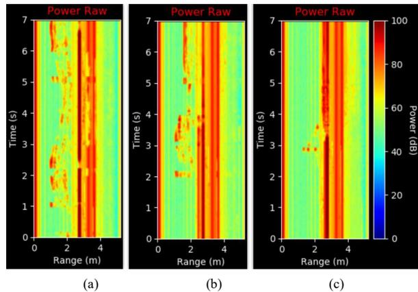
Fig. 2. Example of range-time-power heatmaps of three indoor human activities for mmWave band. (a) Walking, (b) Sitting, and (c) Falling
