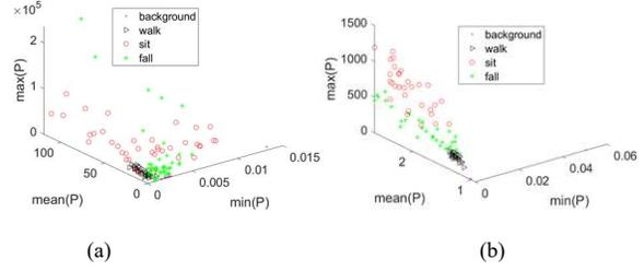
Fig. 6. The distribution of the different classes without using SVD. (a) In mmWave band and (b) in sub-6GHz band
